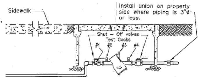
device will fit together, begin connecting all the parts by threading them or soldering them together. Make sure that the arrow on the backflow device is pointing the direction you want the water to flow. Use the union for the final connection.
