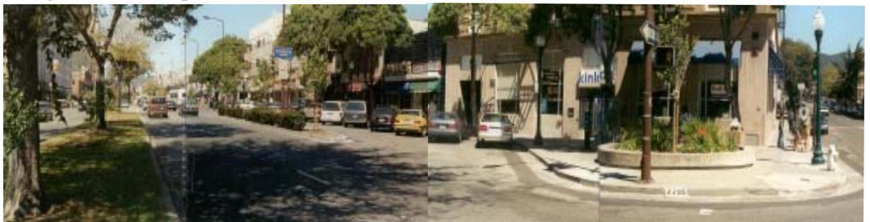
*Fig. 1.3.3 This very wide street in Berkeley, CA, has been reconstructed by replacing travel lanes with diagonal parking in front of commercial buildings to create a very successful streetscape.*
