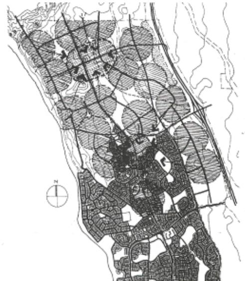
Fig. 1.1.1 This diagram from Western Australia depicts preliminary planning for an area of new growth. It illustrates many concepts fundamental to good Neighborhood Design. New neighborhoods are plotted based on existing constraints and opportunities. They are sized based on a 1/4 mile radius from center to edge. Circulation connects the neighborhood centers.
