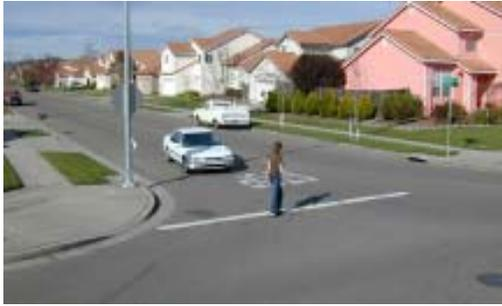
Fig. 1.1.9 36 foot wide street with 25 foot corner radii creates long pedestrian crossing and encourages speeding.
