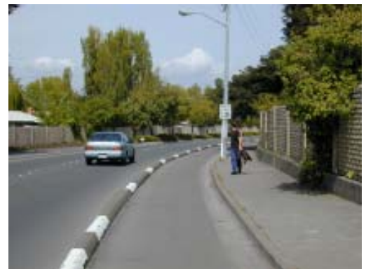
Fig. 3.1.5 Back-on treatment with sound walls should be avoided. They create inhospitable pedestrian environments and encourage traffic to increase speeds.
